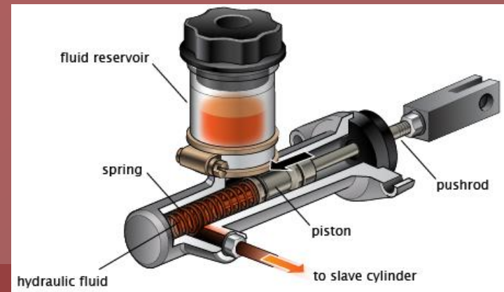
Figure 4-10b Hydraulic clutch linkage
